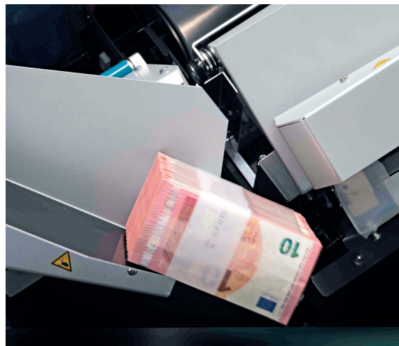
Top: output of bundler delivery modules
